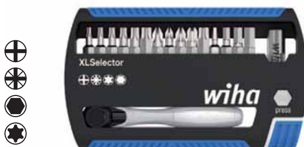
7948-043 XLSelector Torsion, mixed, with 1/4" bit ratchet, 17-pcs. Housing: Box made of high quality plastic. Contains 15 bits, bitholder and bit ratchet. Bits: 25 mm Z and ZOT bits. Geometry: Patented torsion zone to prevent premature breaking of the bit when under stress. Bit holder: 1/4" universal holder, magnetic. Application: Universal assortment for all types of fastening in trade and industry. More applications with practical bit ratchet. Extra: 1/4" universal holder can be used as an extension.
